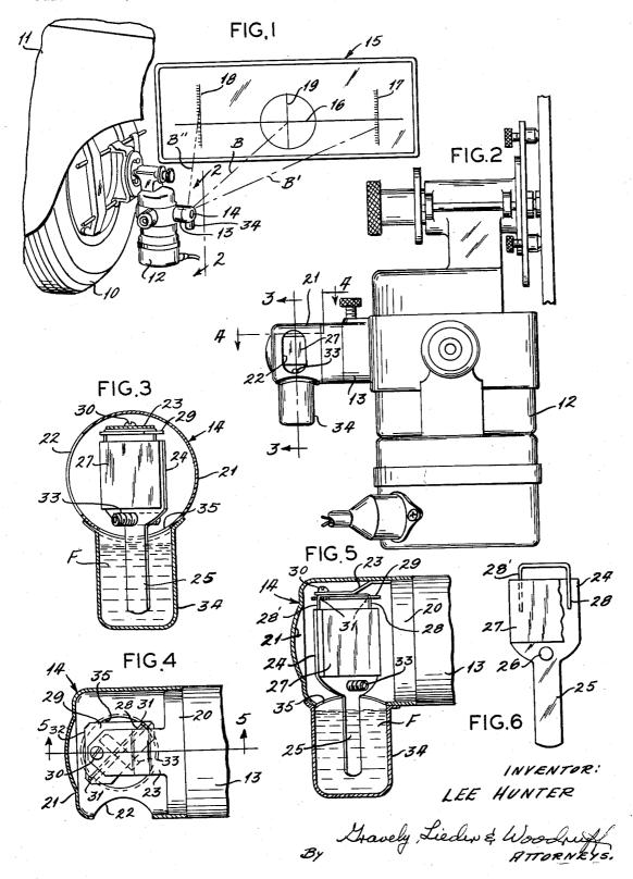
MIRROR MOUNT FOR WHEEL ALIGNMENT APPARATUS
