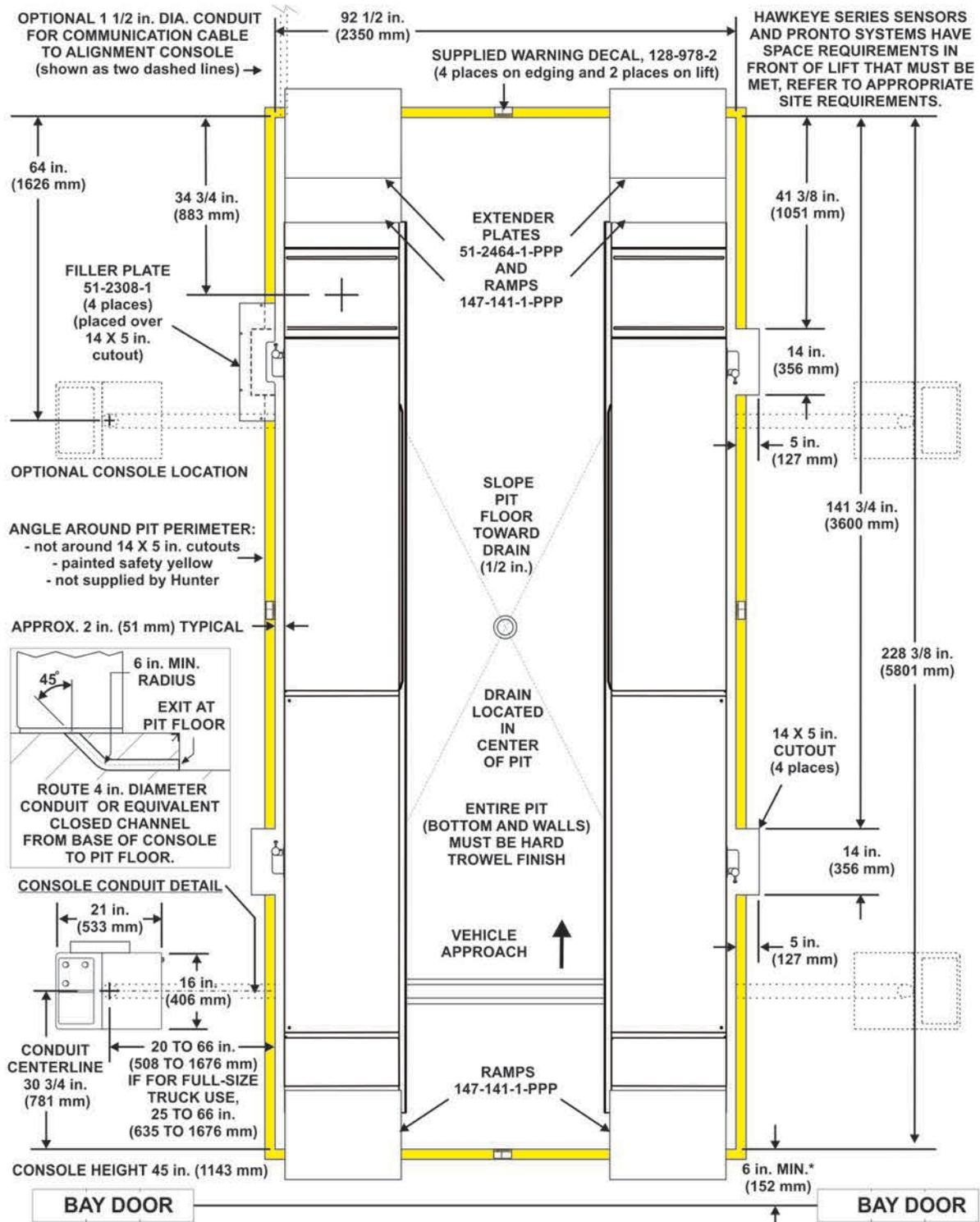
\* LONGER VEHICLES WILL NEED TO BE SERVICED WITH THE BAY DOOR OPEN. TO ACCOMMODATE MOST VEHICLES, INCREASE THE SPACE BEHIND THE PIT TO 39 in. (991 mm) OR GREATER.
