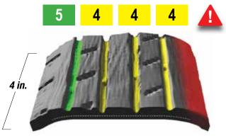
Accurate tread depth calculated for each groove.
